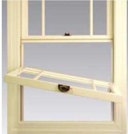
Next, tilt the top sash using the same technique described in **Ultimate Double Hung and Single Hung Windows - Tilting the Sash**. When the sash is in a horizontal position, lift both sides upward 2-3" (raising pivot pins out of each clutch). Finally, rotate the sash until the pivot pins clear the jambs and remove the top sash from the frame.
